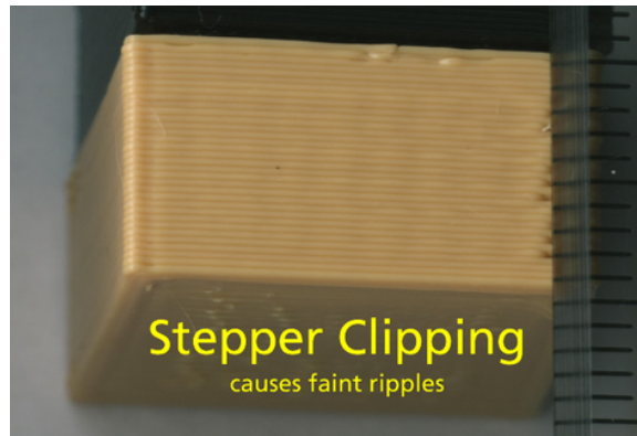
Figure 5.4: Faint ripples caused by stepper clipping
